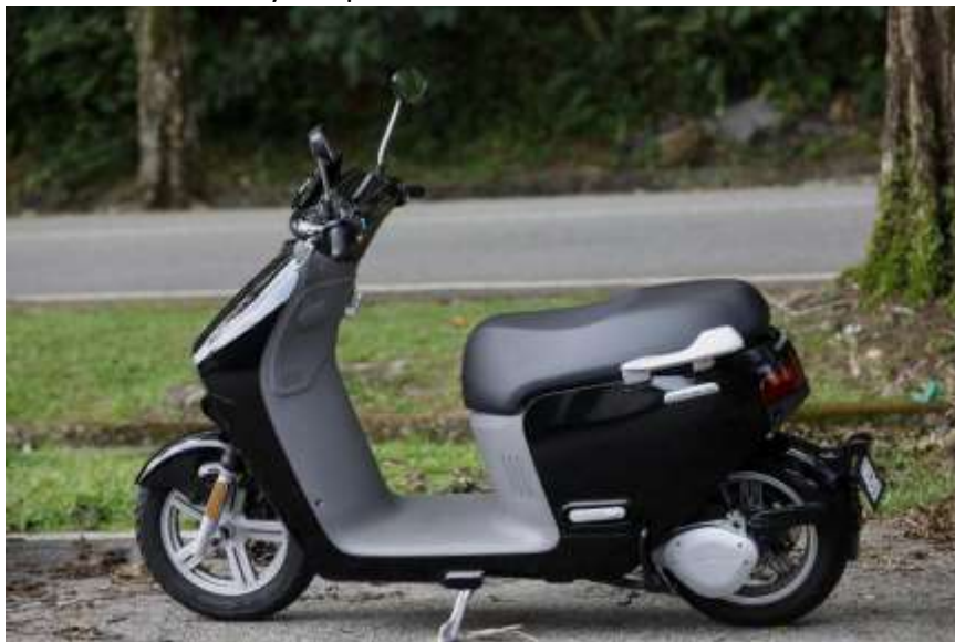
Figure 4 : BlueShark R1 is a step-through frame electric motorcycle with under-seat batteries. Image: CarSifu.my
