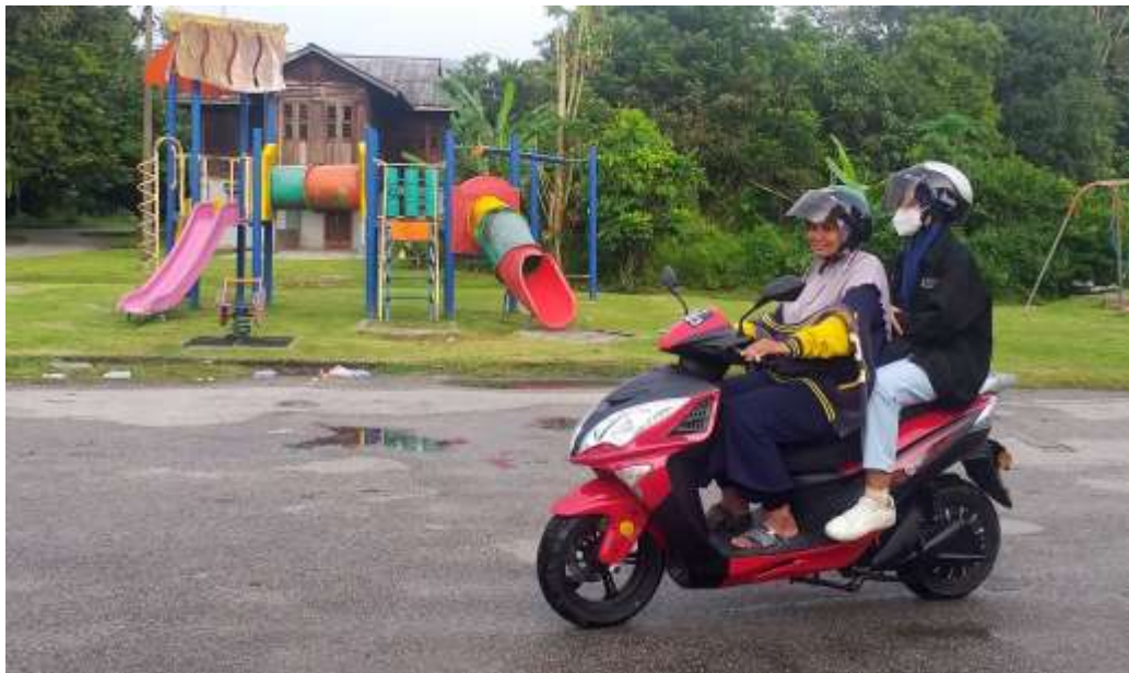
Figure 30 : The rear seat passenger doesn't have a foot peg, causing leg fatigue on even moderate rides
